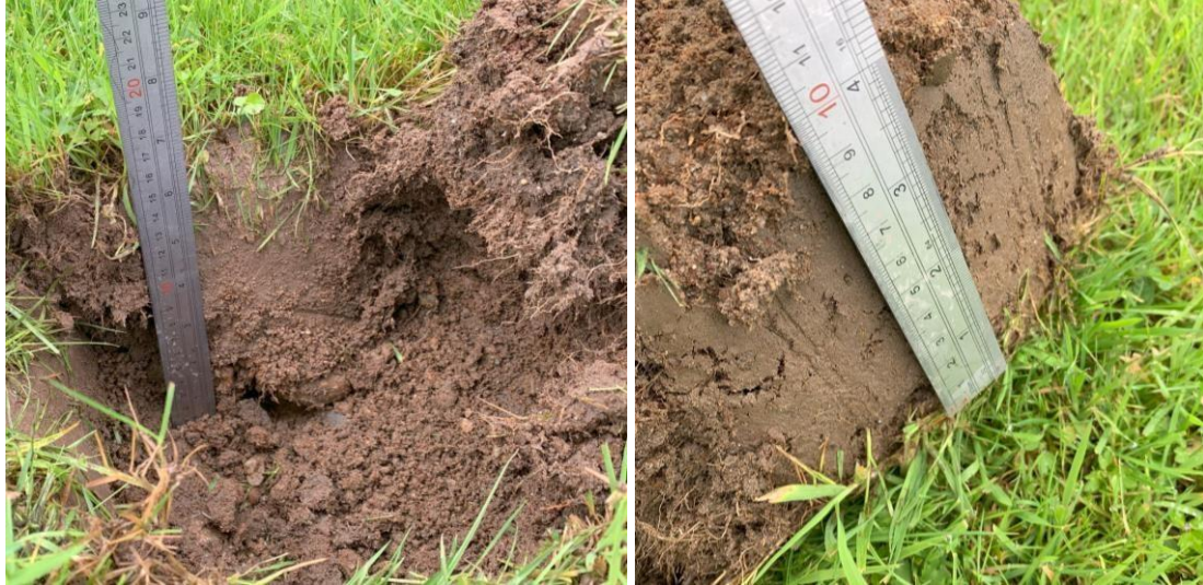
Trial Pit 1 – 160mm of loamy topsoil over a drain run with fine gravel permeable fill. Compact 100mm upper layer with limited root depth, hard subsoil.
